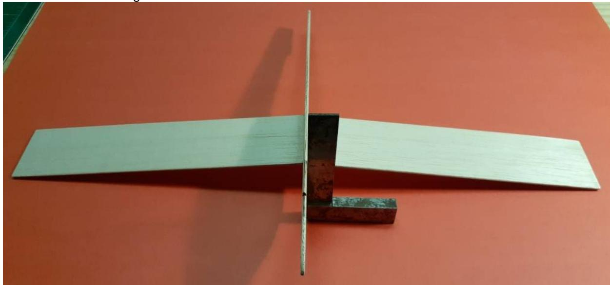
To check this, you can set the fuselage and wing inverted on a flat surface. Use a right angle to set the fuselage vertical. When satisfied with the alignment, run thin superglue along each side of the joint to glue the wing in place. Glue on the top surface when the glue is set.
