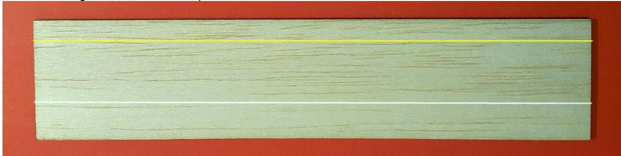
Take your sanding stick and sand the top front edge of the wing in a curve down to the bottom edge. Start this about 3/8" (9mm) back from the front edge (yellow line). Then round the bottom corner of the front edge. Do this along the whole length of one wing panel.
