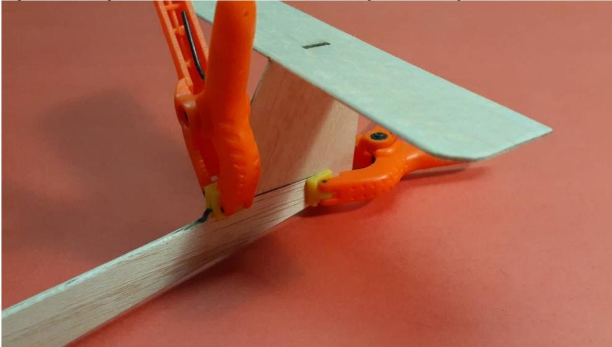
You can use small spring clamps to hold the tail fin in position. When you are satisfied with the fit, glue the assembly onto the fuselage. Make sure that the fin is vertical and exactly in line with the fuselage center line.
