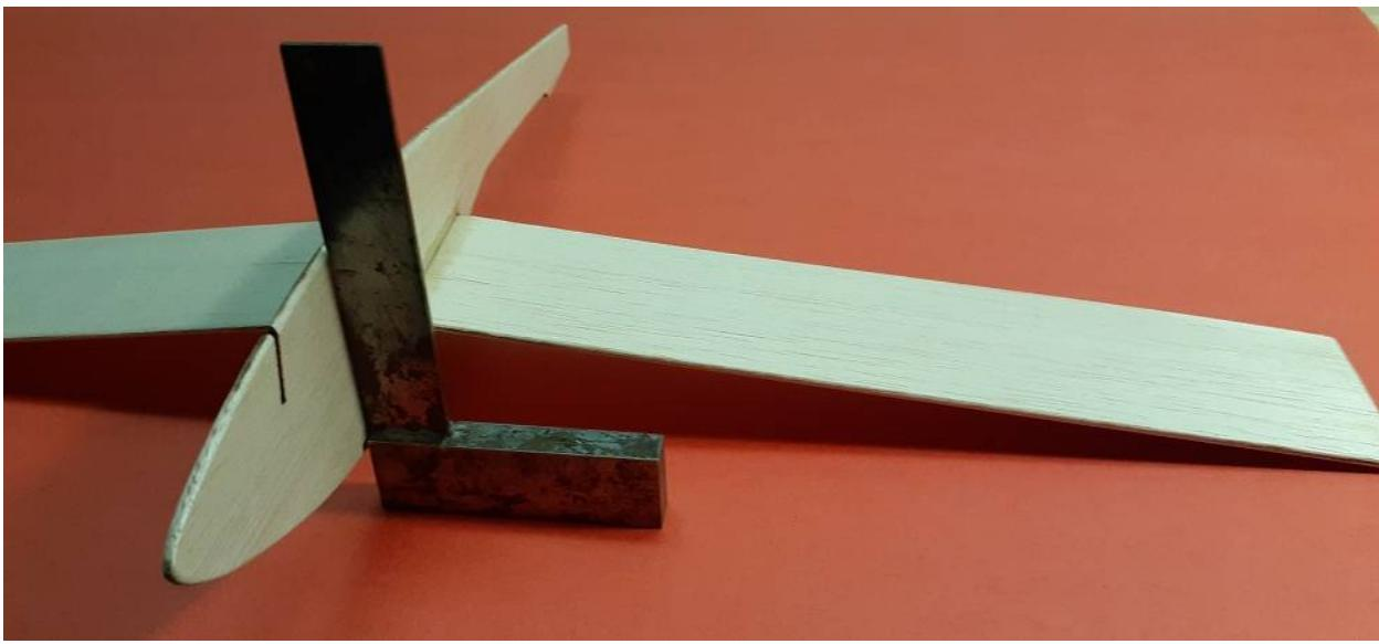
Slot the tailplane onto the tab on the tail fin. Set the pieces on your building board and use a right angle to get the fin at 90 degrees to the tailplane. Glue in place with superglue.
