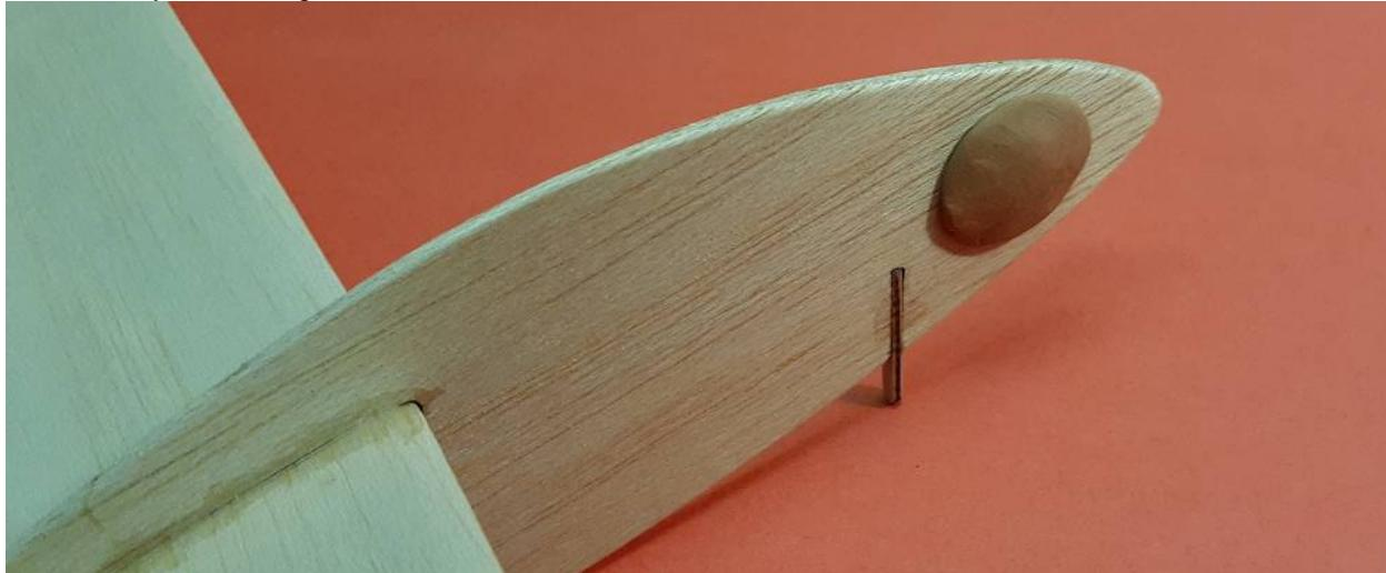
Throw the glider with the wings level and the nose slightly down. Try to throw it just fast enough for it to glide away from you steadily. If the model dives downwards, remove a little clay. If the model climbs and then dives (stalling), add a little more clay. Aim for a slow glide with a nice smooth flight.
