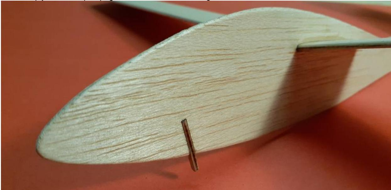
If you are building the version with the wing tip mounted fuel tanks, add them next. The wing tip tanks slot onto the end of each wing. When gluing in place make sure that each is exactly in line with the end of the wing tip and parallel to the fuselage side..
